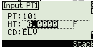
Fig. 9.21: Point Input Screen (PT1)
